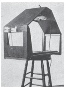
**Depth perception -** The modification to the depth perception tester pictured here kept applicants from looking over the top and also reduced glare and removed shadows from within the apparatus.
