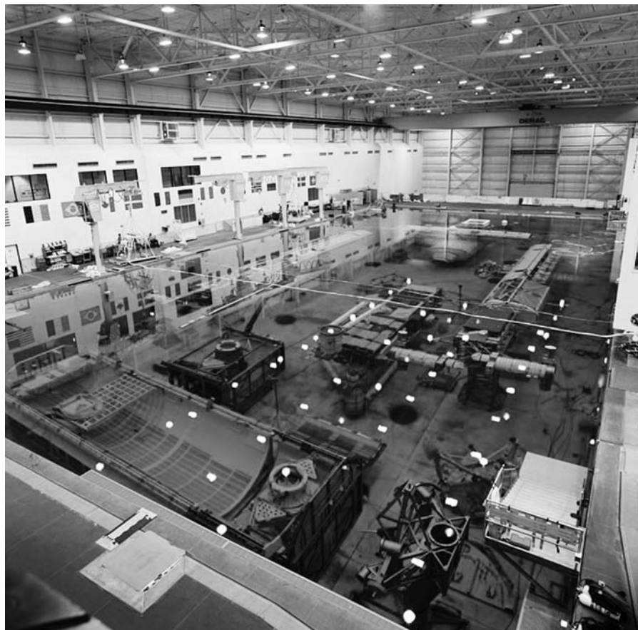
Fig. 2. The NBL configured with mockups of the Space Shuttle cargo bay and the International Space Station.
