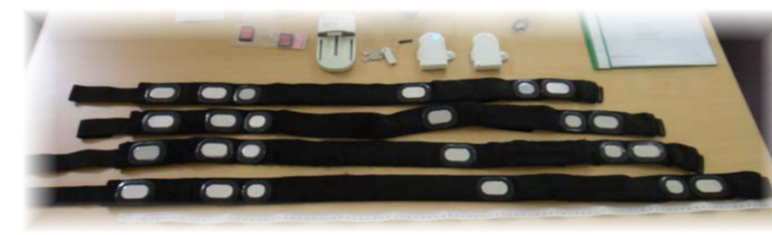
Fig. 5: Chest belts with integrated electrodes for ECG and thorax impedance recordings.
