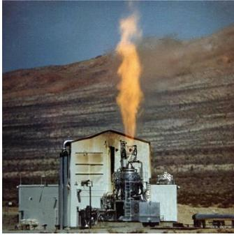
*Kiwi A nuclear rocket engine test. (Los Alamos National Laboratory)*
