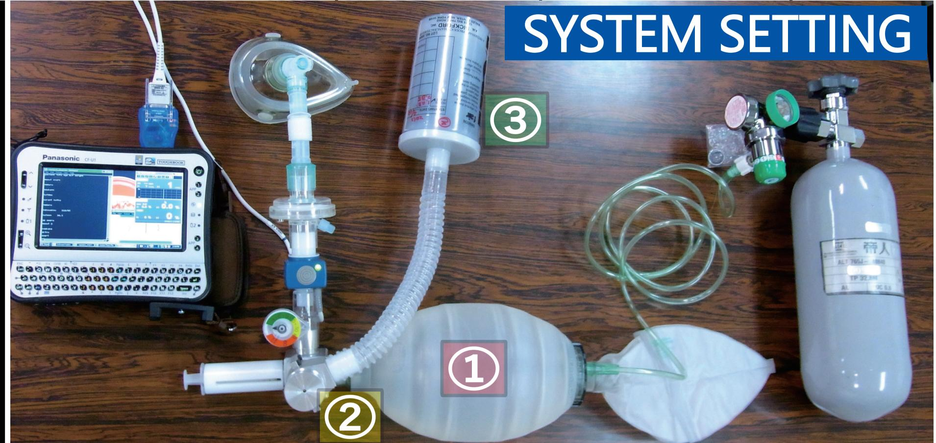
A new 3D printable device was invented which, by fitting to a conventional bag valve mask (BVM), allows the addition of 3 KEY functions of inhaled general anesthesia systems:
