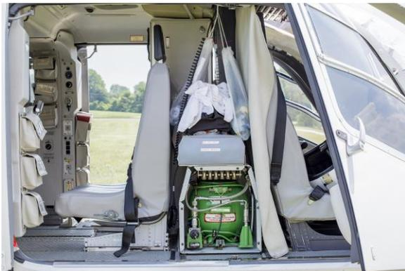
Essex LOX converters for air medical transport are available in 5, 7 and 10-liter sizes. Essex also offers the Ready to Install (RTI) LOX system. The RTI consists of a 10-liter LOX converter with a heat exchanger and regulator mounted inside a sheet metal enclosure. This configuration allows installation of the equipment on aircraft without the expense of a costly retrofit. The 10-Liter LOX Converter supplies up to 8,600 gaseous liters of
